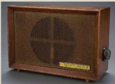
Photo of a Rediffusion box (loudspeakers with a built-in amplifier)
